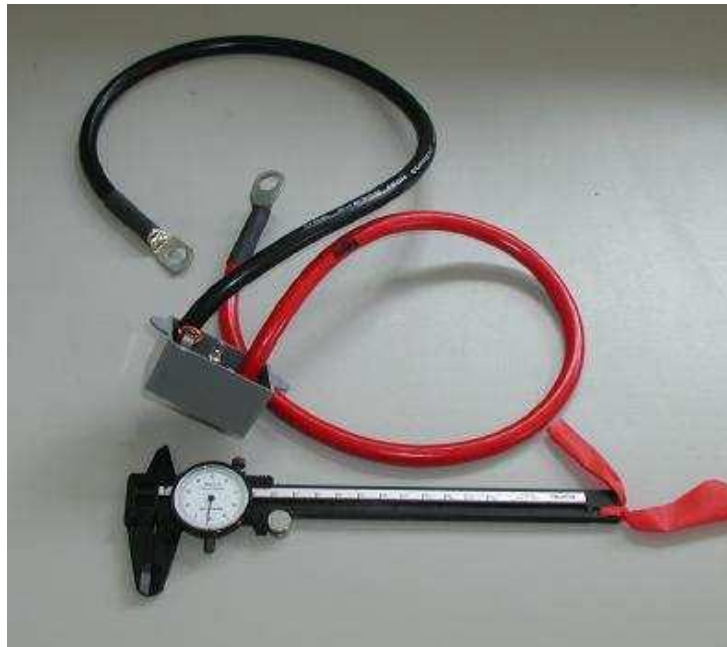
Fig 10 Packaged de-sulphator, ready for installation. Caliper is 230 mm long. Note heavy high current wires.
