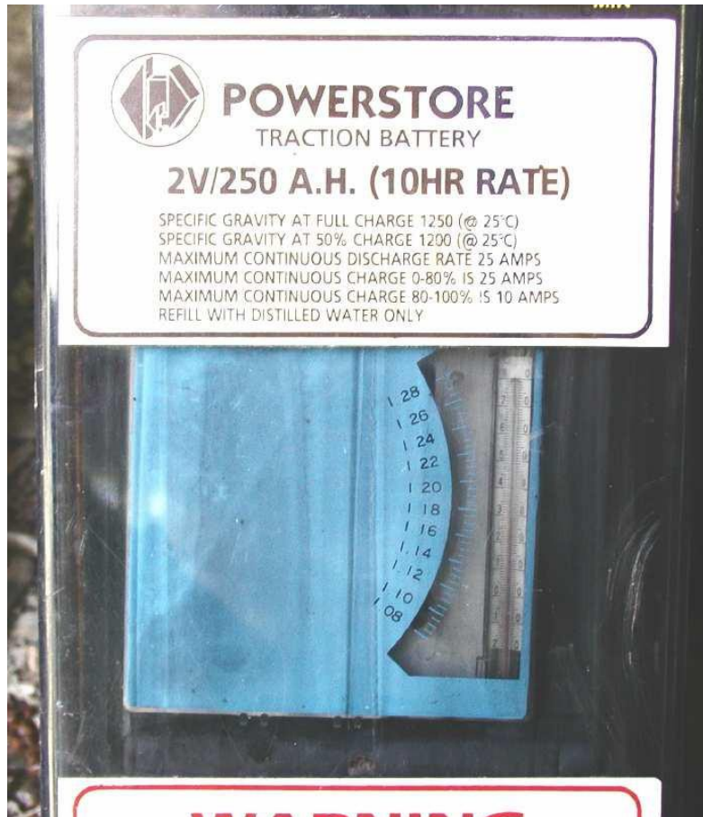
Figure 1 Built in hydrometer and thermometer in a Australian made tubular plate cell. The unit (Japanese made) is simply inserted between the plate array and the side of the case.
